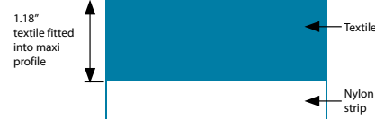
Application of nylon strip by double sided tape
