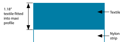
Application of nylon strip by double sided tape
