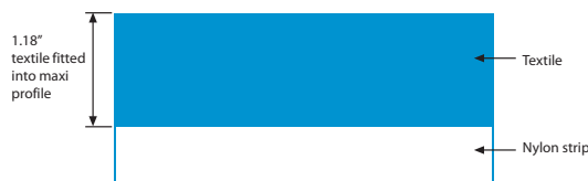
Application of nylon strip by double sided tape
